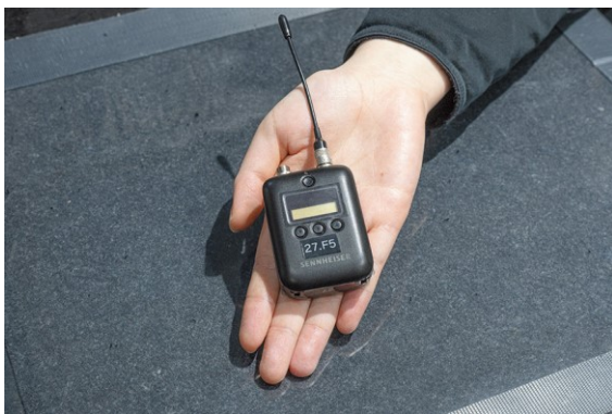
The SK 6212 mini-bodypack transmitter is small and lightweight, and therefore easy to hide
